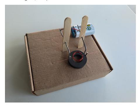
(NOTE: Depending on the power of your magnet and battery, you might need to give the copper ring an initial push to spin it.)
